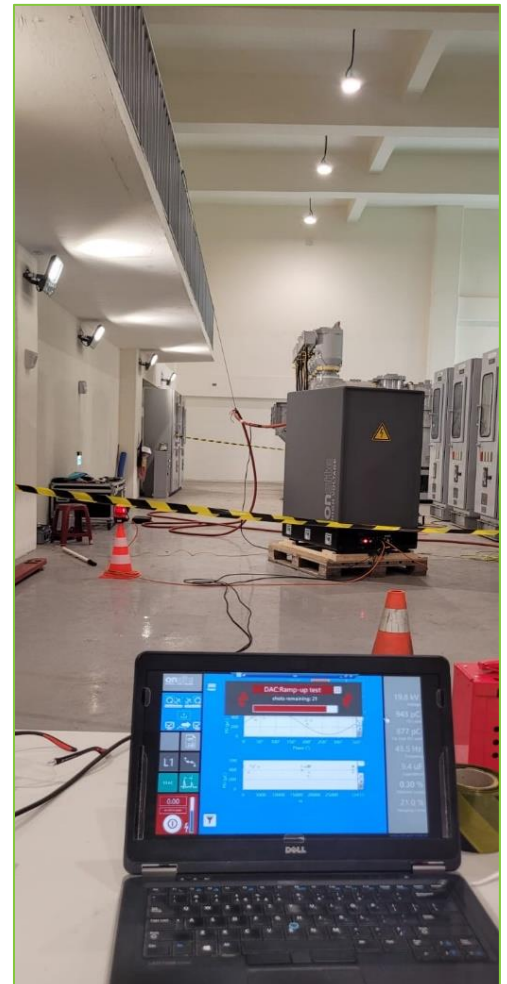
Export cables testing using DAC HV110 system: Master unit with Dual-Power installed on the on-shore substation (on the bottom). Far-end unit with Dual-Side installed on the off-shore substation (on the top)
