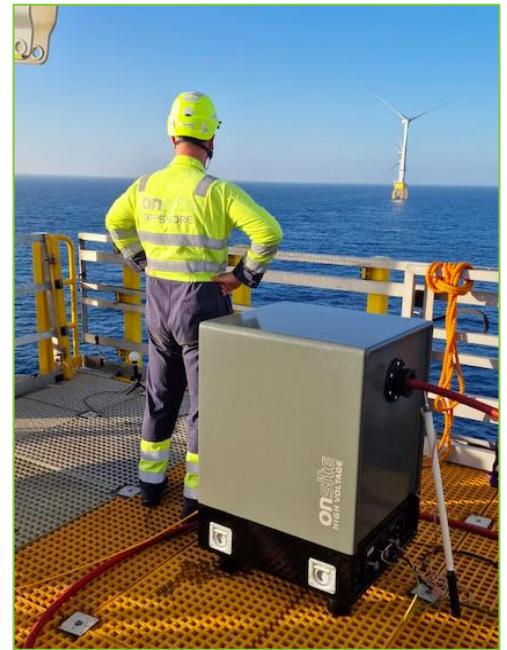
Export cables testing using DAC HV110 system: Master unit with Dual-Power installed on the on-shore substation (on the bottom). Far-end unit with Dual-Side installed on the off-shore substation (on the top)
