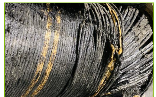
Field examples of mechanical damage on the armour of an inter-array cable
