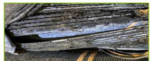
Field examples of mechanical damage on the armour of an inter-array cable
